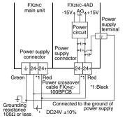
• Connect the " ± " terminal together with the ground terminal of the PLC main unit to the ground of the power supply equipped with grounding resistance of 1000 or less
