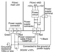
• Connect the "  $\pm$  " terminal together with the ground terminal of the PLC main unit to the ground of the power supply equipped with grounding resist 100Ω or less.
