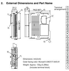
Accessory: Special function block number label, Power crossover cable FX2NC-10BPCB1 2) Terminal connector (European type) 1) Status indicator LED
