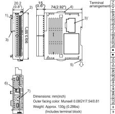
Accessory: Special function block number label. Power crossover cable EX2NC-10BPCB1
