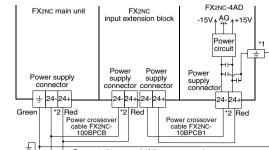
Grounding Connected to ground of the power supply \*1:Power terminal resistance + DC24V ±10% \*2:Black resistance 100Ω or less
