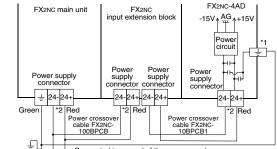
Grounding Connected to resistance + DC24V ±10% Connected to ground of the power supply \*1:Power terminal \*2:Black
