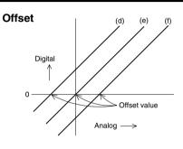
Gain determines the angle or slope of the calibration line, identified at a digital value of 1000.
