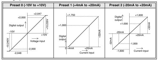
NOTE: Preset ranges are selected by an appropriate setting in the buffer memory of the analog block. Current/Voltage input selection must match the correct input terminal connections.
