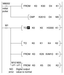
The ID code for the special function block at position "0" is read from BFM #30 of that block and stored at D4 in the main
